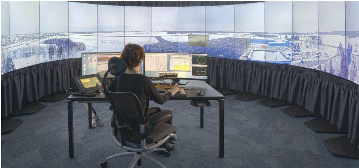
*The remote tower solution from ANSP Estonia Air Navigation Services (EANS) and Cybernetica displaying a view of the airfield at Tartu Airport. (EANS)*
